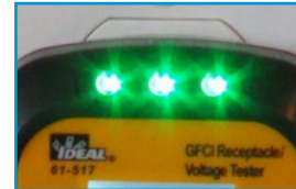
Green Lights Indicate Correct Wiring
