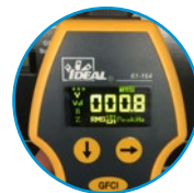
Displays neutral to ground voltage
