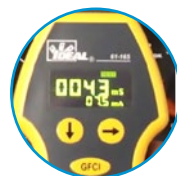
Trips GFCI at 6mA or 30mA
