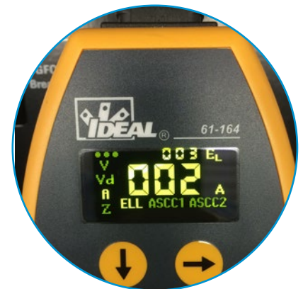
Estimated Load on Line in Amps
