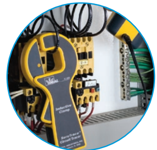
Inductive Clamp for when direct contact with alligator clips is not possible
