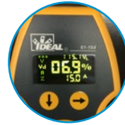
Displays Voltage Drop at 12, 15 & 20 Amps
