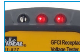
Red Lights Indicate Incorrect Wiring
