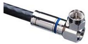
6) Verify connector is fully compressed. InSITE™ window is no longer visible and connector is now shorter in length than an uncompressed connector.
