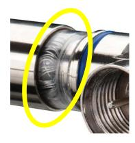
4) Cable is fully seated when braiding is visible in the clear InSITE™ window.
