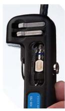
5) Adjust compression tool post for right angle connectors by lowering threaded post to bottom line marker with a flathead screwdriver. Place assembly in compression tool (30-793 shown) and compress. Connector compresses against the top level spring clips.
