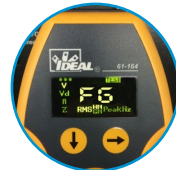
Detects and Displays false or "bootleg" ground
