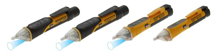
61-657 Dual Range 12 to 1000V AC NCVT w/Flashlight CAT IV 1000V **61-647** Single Range 50 to 1000V AC NCVT w/Flashlight CAT IV 1000V **61-637** Single Range 24 to 600V AC NCVT w/Flashlight CAT IV 600V 61-627 Single Range 50 to 600V AC NCVT CAT IV 600V
