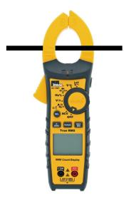
**Safety** - A clamp meter allows you to measure AC or DC current (depending on the model) by positioning the clamp jaw around a conductor, which is much safer than making direct contact with a live circuit.
