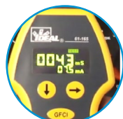
Trips GFCI at 6mA or 30mA
