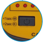
On/Off Button Confirms Tester is Working
