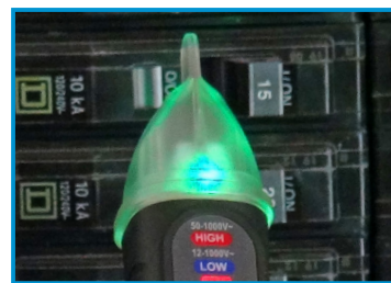
Power On Indicated by a Green LED
