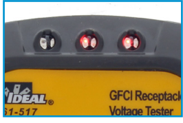
Red Lights Indicate Incorrect Wiring
