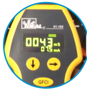
Trips GFCI at 6mA or 30mA
