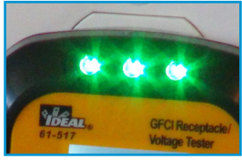
Green Lights Indicate Correct Wiring
