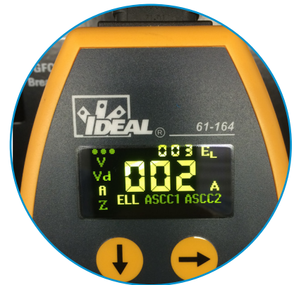
Estimated Load on Line in Amps
