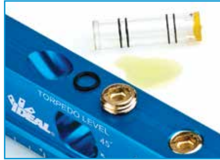
2. Remove O-ring and damaged vial
