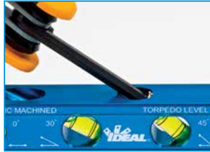
4. Reinstall O-ring and set screw
