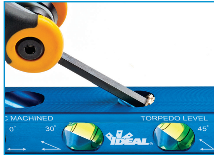
1. Remove the set screw with hex wrench
