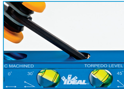
4. Reinstall O-ring and set screw
