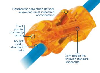
SpliceLine® in-line wire connectors provide a crimpfree, solderless butt splice. Accepts a broad range of wire sizes, allowing one connector to do the job of multiple through-crimps. Its end-to-end connection is also a great solution for pre-fab operations
