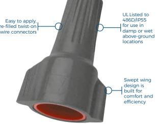
Designed specifically for above ground, interior/exterior connections exposed to damp/wet and corrosive environments. WeatherProof connectors are pre-filled with a non-hardening, silicone-based gel that protects against moisture and corrosion.
