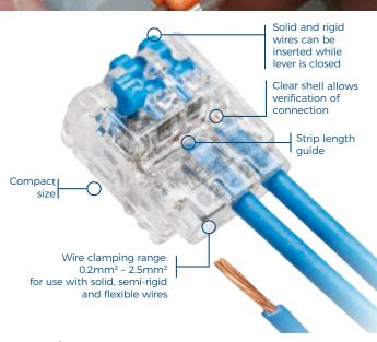
In-Sure<sup>®</sup> lever wire connectors provide the perfect solution for joining solid, stranded or flexible conductors.
