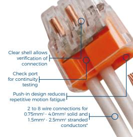
In-Sure<sup>®</sup> push-in wire connectors reduce installation time by up to 50%. They are the perfect replacement for traditional terminal blocks. The popular 2, 3 & 4 port models are rated to 32 Amps.
